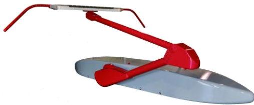
Single-Arm Pantograph for High Speed Train
