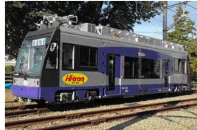
Toyo Denki supplied converter units, drive inverter units, auxiliary power supply apparatus, gear units, traction motors, and pantographs for the hybrid light rail vehicle (LRV) unveiled by the Railway Technical Research Institute
