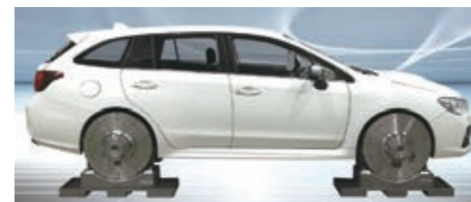
Actual vehicle test with in-wheel-well dynamo
