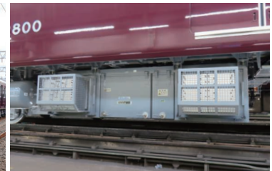
Exterior of the Propulsion controller (VWF inverter) (photo provided by Hankyu Corporation)
