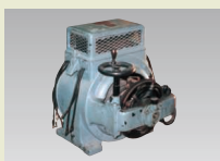
Three-phase current commutator motor (Schrage-type, later AS motor)
