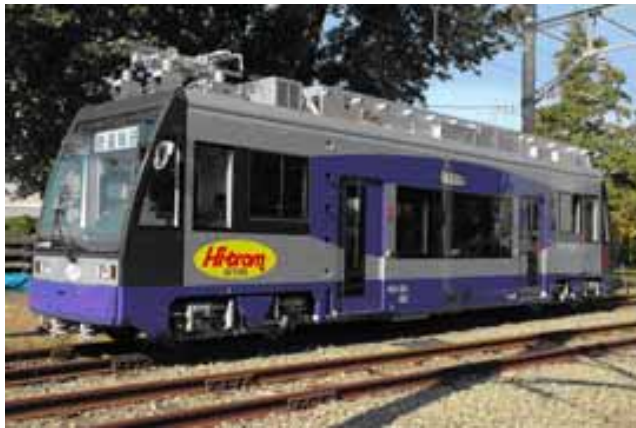
Running on batteries (Without pantograph)
