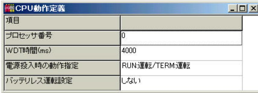
There are 3 setting items in the CPU operation definition: watch dog timer, explanation of operation at the time of powering on, and operation without batteries.
