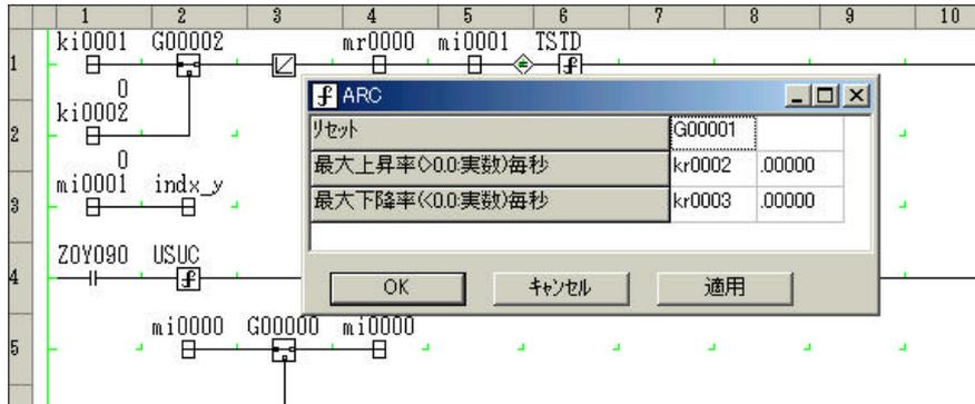
After closing the argument setting window, it can be displayed by double clicking on the function symbol.
