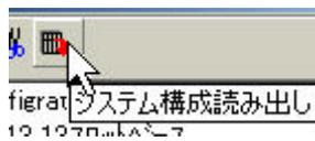
When being on-line, it reads the system configuration information from the  $\mu$  GPCsx. The conditions can only be read on condition that the  $\mu$  GPCsx is not in a serious failure.
